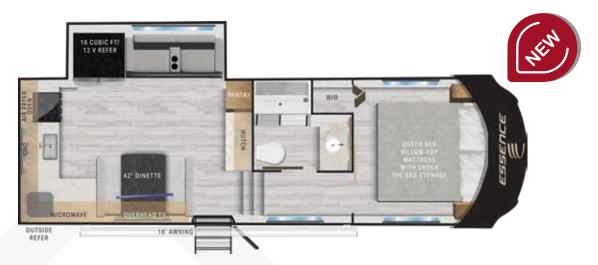
Overall Length: 28-11" GVWR: 10,000 LBS Dry Weight: 7,808 LBS Hitch Weight: 1,372 LBS Axles: 2×5100 Fresh Tank: 96 Gal Grey Tank: 87 Gal Black Tank: 30 Gal Furnace: 35,000BTU A/C: 15,000 BTU Main Slide Height: 6´-6″ Bedroom Height: 6´-4″ Awning Length: 16´ Refrigerator: 16cu/12V
